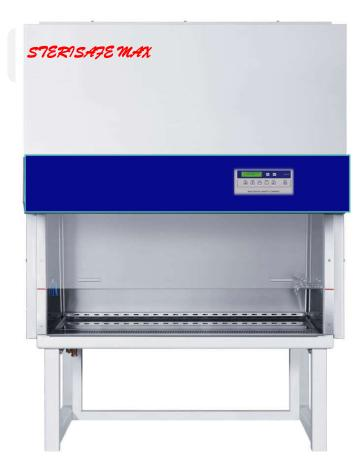
Three sides of the inner wall are all stainless steel and adopt integrated structure, 12mm big circular arc filtration can do complete washing.
